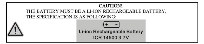
To install the battery for the first time, please make sure the unit is not connected to AC power. Install the battery in the battery holder, then remove the battery and install it back. This procedure must be done only for the first battery installation.
